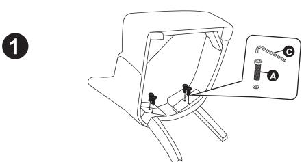
Put the screws in the holes, tight the screws, but not too tight, 90% is ok.
